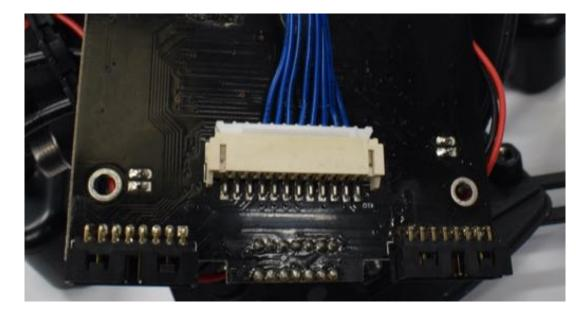
6. Flip the board back over, threading the cable as shown.
