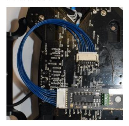
16. Place a cable tie base onto the PCB and cable tie the 8 blue cables to keep all cables clear of the rear metal piece which will come over the top.
