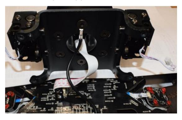
14. Find a suitable place for the conversion circuit board and fix onto the main PCB. Our chosen location is shown below. Make sure that you give the PCB enough clearance from the metalwork, which will cover the PCB.
