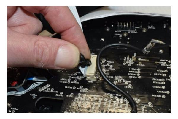
8. When all the glue is removed, pull the connectors apart. To avoid pulling the entire connector off the board, use both hands. One on the PCB connector, and one on the cable connector. I used my left hand to pull on the cable connector, and my right hand to hold the connector on the PCB.
