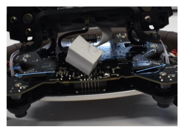
I found it best to use some long nose pliers and taking my time. When this is done, pull the rear part of the wheel away from the front and place on some protective paper or card as shown.
